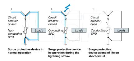
The disconnecting device must be coordinated with the surge protective device. It is designed to meet the following two constraints:
