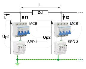
L and Zd represent the cable length and impedance respectively between the 2 surge protective
